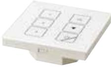
DALI TOUCHPANEL BASIC performs a variety of lighting tasks in small and medium-sized rooms such as offices, hotel rooms, classrooms and meeting rooms and is very easy to use. Luminaires can be switched on and off, dimmed and grouped via the control panel with six individually assignable keys. DALI TOUCHPANEL BASIC is available in the four layouts COMBINATION, GROUP, SCENE and TUNABLE WHITE.
