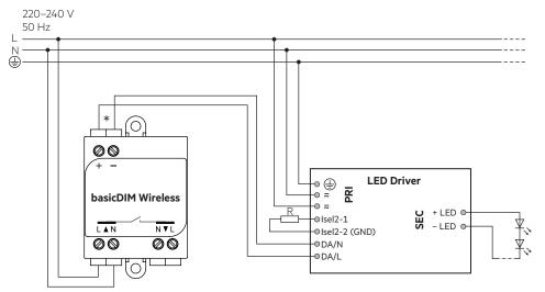
$^{*}$  Max. wiring length 1 m with a cross section of 1 mm<sup>2</sup>.
